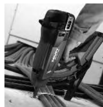
Conduits & pipes with metal or textile band
