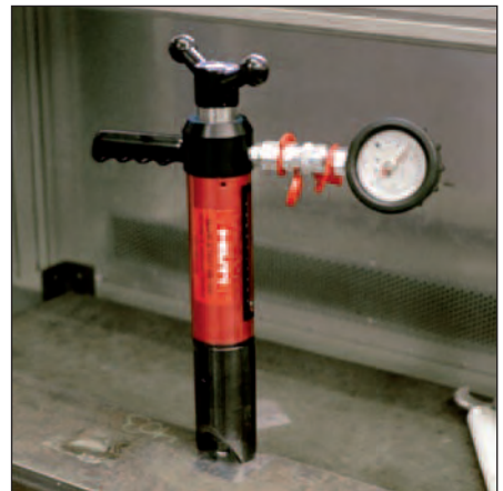
Pull-out test of an ENP fastening with a Mark V tester and ENP adapter
